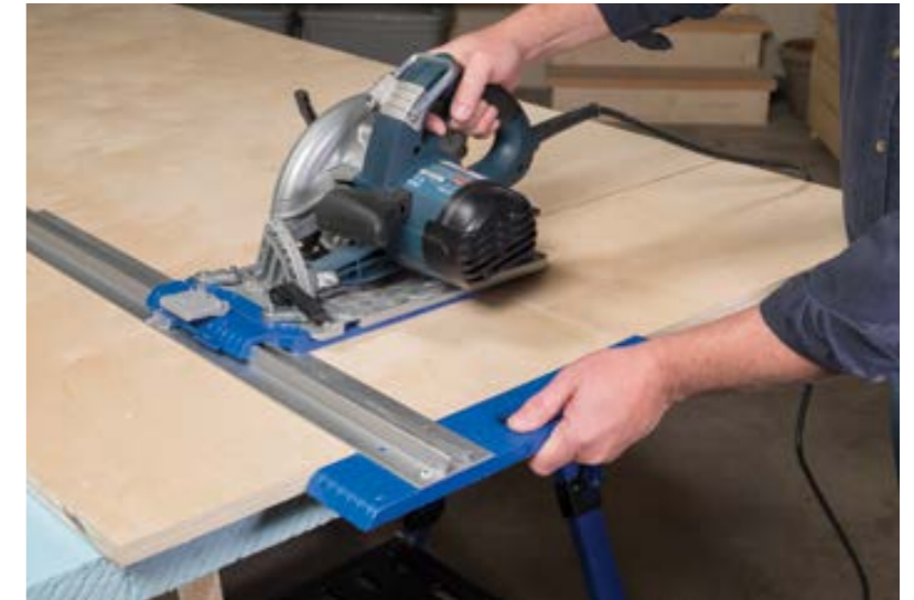
Make cuts wherever you want to by taking your saw to the workpiece rather than taking your workpiece to the saw.
