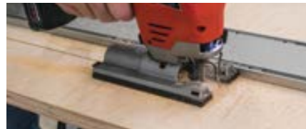
Aluminum guide rail leads cuts precisely along a straight line
