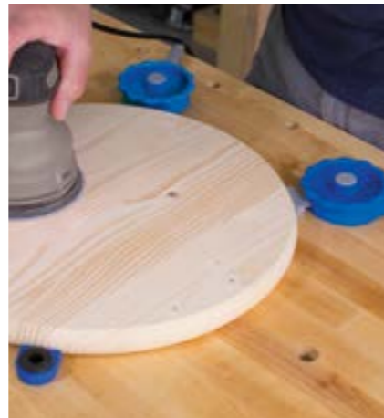
Clamp shoe holds flat and rounded shapes, as well as 90°.
