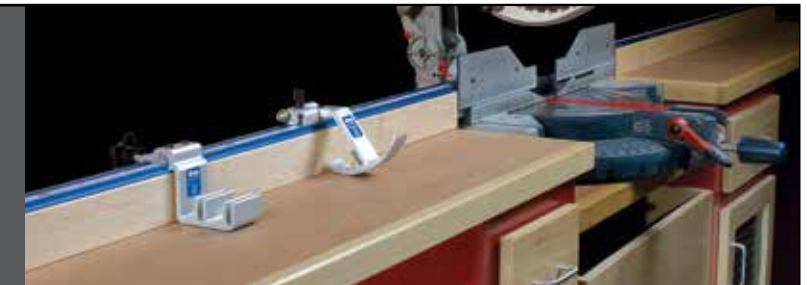
Center your saw with 4 feet (1220mm) of Trak on each side.
