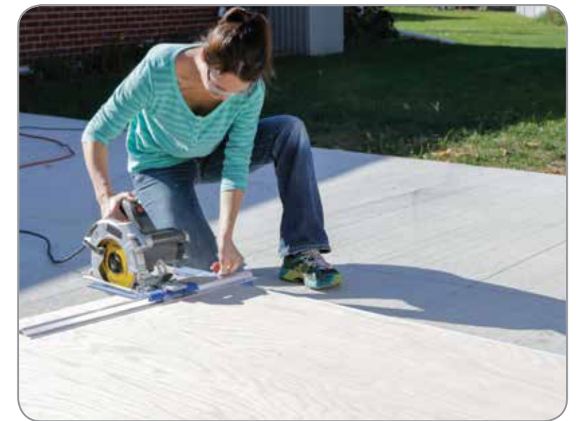
The Rip-Cut™ makes it easy to achieve straight, accurate, repeatable cuts using an ordinary circular saw.
