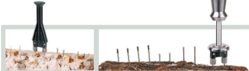
**APPLICATION** Overview over various pin length: Use in conjunction with M 20 [left-hand side] and M 18 [right-hand side] electrodes
