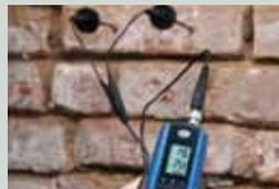
**APPLICATION** Measurement of **structural moisture in bricks** using an M 25-100 brush electrode pair [left-hand side] and **measurement of plaster moisture** using an M 20 electrode [right-hand side]
