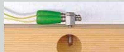
**APPLICATION** Connecting **non-insulated** [above] and **insulated** drive-in electrodes [below]
