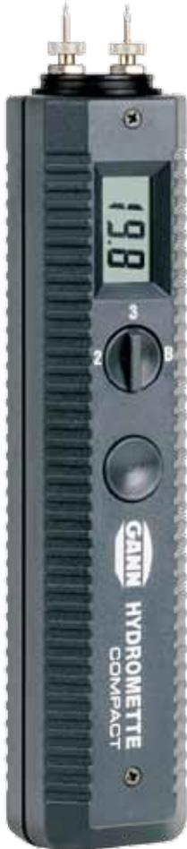
The Compact unit is an electronic **wood and plaster moisture meter** that uses the resist-ance principle of measurement.
