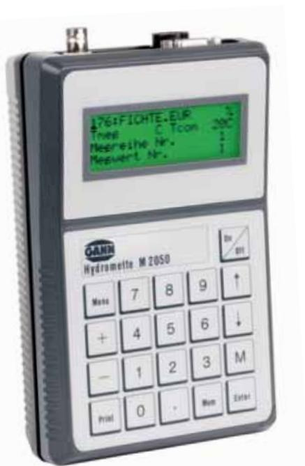
The M 2050 unit is an electronic **wood moisture and temperature meter** that is based on microprocessor technology and provides **measured data storage** as well as connectivity to a PC or printer.
