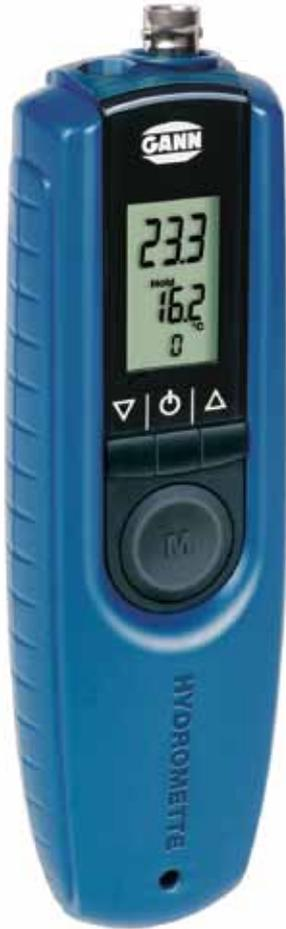
The BL E unit is an electronic **structural moisture and temperature meter** for precisely measuring **building and insulating materials**. The unit is based on the resistance principle of measurement and is used for individual measurements. The unit has a material selector for directly indicating the structural moisture in % of 23 building and insulating materials such as screeds, mortars, plasters, concrete, bricks, and a number of other insulating materials.
