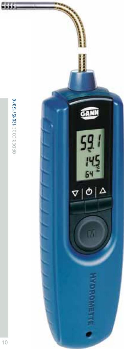
The BL Compact RH-T FLEX 250/350 unit is a **precise thermo hygrometer** designed to be used for quickly measuring the relative **humidity** and **temperature of the air**. Using programmed **sorption isotherms**, the weight and mass percentages can be determined for various building and insulation materials, as well as for hardwood and softwood.
