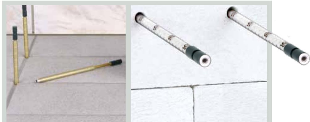
**DETAIL** Both electrode pairs are equipped with one-centimetre division scale
