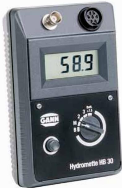
The HB 30 unit is an electronic **wood and structural moisture meter** that uses the resistance principle of measurement for precisely measuring **sawn timber** (up to 180 mm in thickness), **chipboards, parquet, and set building materials**.
