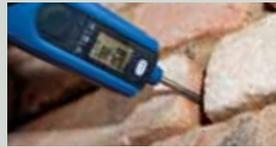
**APPLICATION** Moisture measurement using **sorption isotherms** for quantitatively assessing damage caused by moisture
